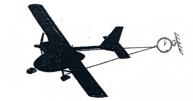
Fig. 2 Propeller static thrust check up.
