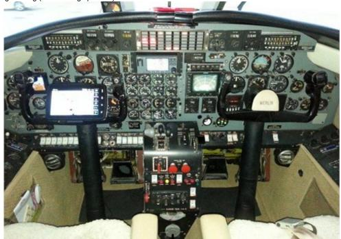
AVIONICS: ADS-B Out Comms: Garmin GTN-650; Garmin GTN-750 GPS: Garmin GTN-650; Garmin GTN-750 Navs: Garmin GTN-650; Garmin GTN-750 Emergency Locator Transmitter Garmin GPS-400W WAAS GPS Navigator M-4D Autopilot w/ Flight Director & Yaw Damper
