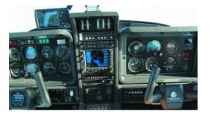
Modular panel has right-side gauges angled to face the pilot.
