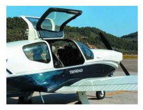
The door sill is higher than on a Piper or Beech, but the large opening helps ease boarding.
