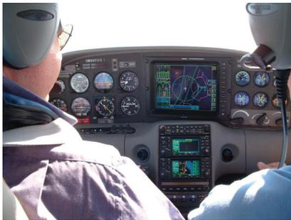
Other standard equipment included a Garmin GNS430 GPS/Nav/Comm, a GNC-250 GPS/Comm, and an S-TEC 20 autopilot. Options included a Century HSI and 3-blade prop, dual alternators, Stormscope, and an
