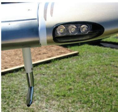
Other improvements include wingtip recognition lights, increased airflow in the environmental systems, redesigned gear and wing fairings, and a taller landing gear for better prop clearance. There was no change to the 3,400-pound maximum gross weight limit, although the CG
