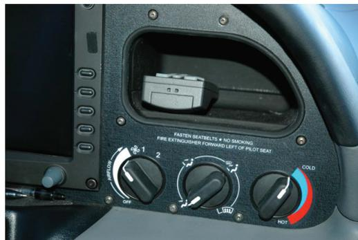
Finally, excellent car-like climate controls were added along with improved air flow. The fan-forced ventilation option was a very nice feature in the greenhouse cabin of a Cirrus without air conditioning - taxiing with the doors open was no longer standard procedure. A second "flight time" meter was installed alongside the Hobbs meter (SR22 Serial #1863, SR20 #1639).
