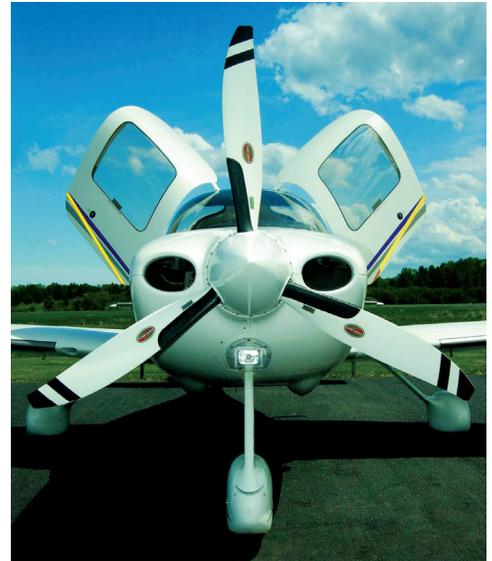
Generally Cirrus owners report the SR22 G2 to be three to four knots faster than its predecessor ... but unfortunately the TKS system installed on most has a drag penalty that pretty much cancels out the gain. As a result, a G2 with TKS is about the same speed as the original SR22 without the TKS panels
